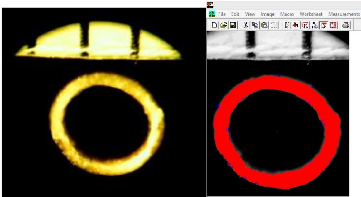
Figure 4. Image of wheat straw under microscope and being analyzed with SigmaScan 5 software.
