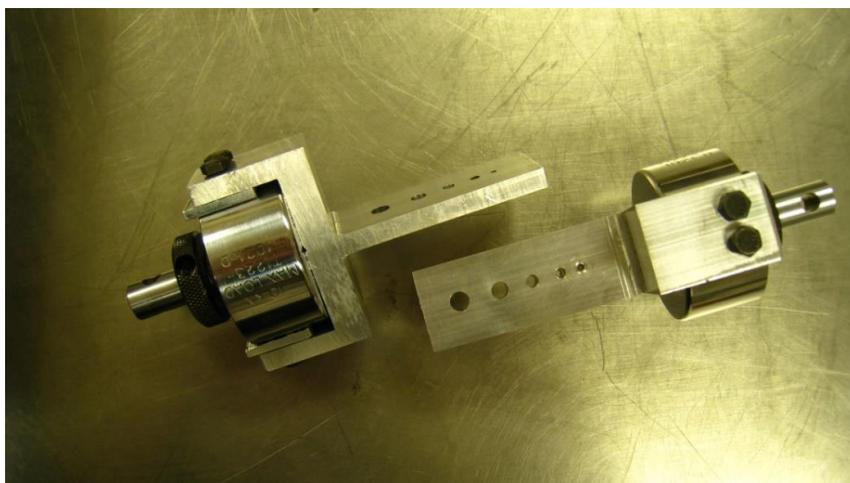
Figure 1. Design of shear box in AutoCAD 2010 and manufactured shear box.
