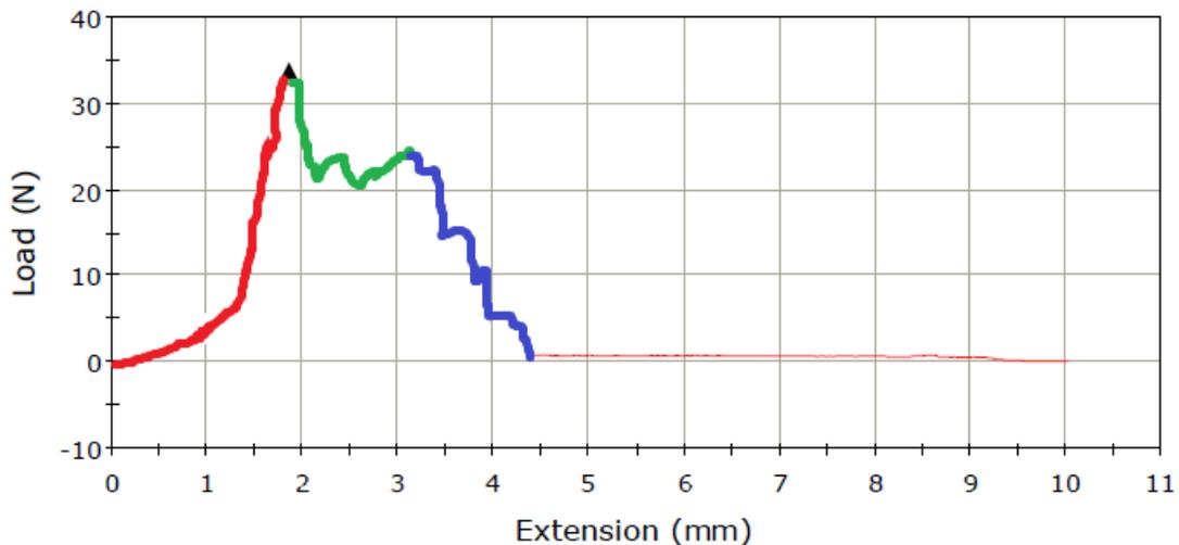
Figure 3. Shear force verses blade extension recorded by computer with different colors showing different shearing stages.
